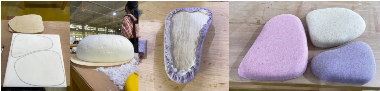
Fig. A4. The process of making seat cushion soft packs. (Source: From this study)
