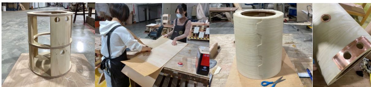
Fig. A2. Air tank manufacturing process (Source: From this study)
